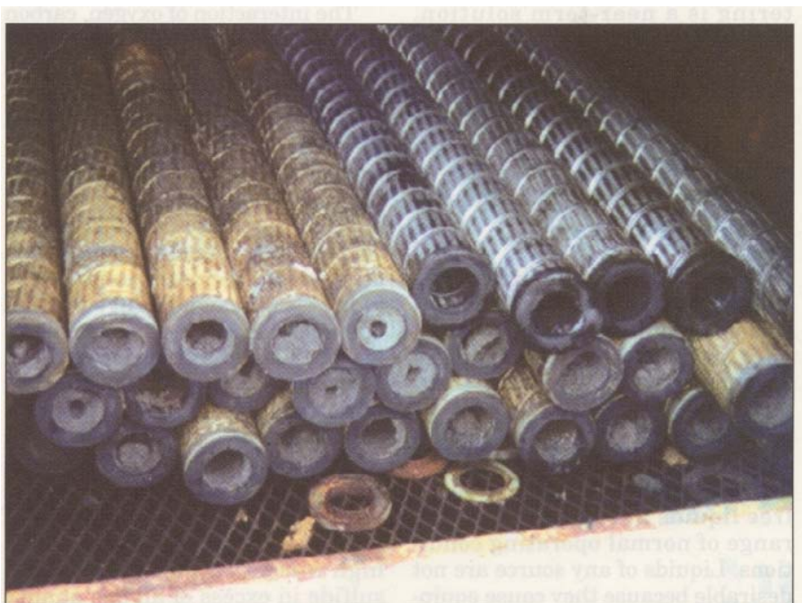
Filtering black powder. From an overview perspective of the black powder problem, filtering is a near-term solution; however, it is a superficial or local spot solution and would be less demanding and less expensive if the source of the gas were properly treated to eliminate iron sulfide formation.
