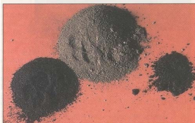
What is it? Black powder is a catch-all term that describes material that collects in gas pipe lines and creates wear and reduced compressor efficiency, clogged instrumentation and valves, and
